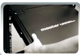
2. Slide the LCD KVM Switch / LCD Console onto the rails and secure it to the rack.
