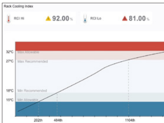
eco DC: Overall Rack Cooling Effectiveness
